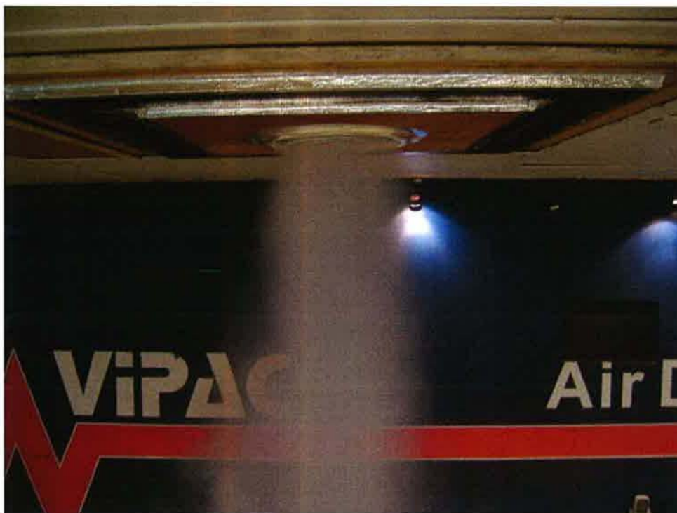
Figure 9: Jet Ceiling Diffuser (Neck: Ø245mm).
